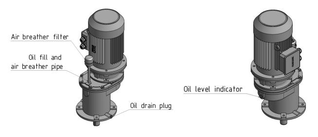
Oil level indicator, breather filter and pipe and oil drain plug should be reachable at all times for regular controls and maintenance activities.
